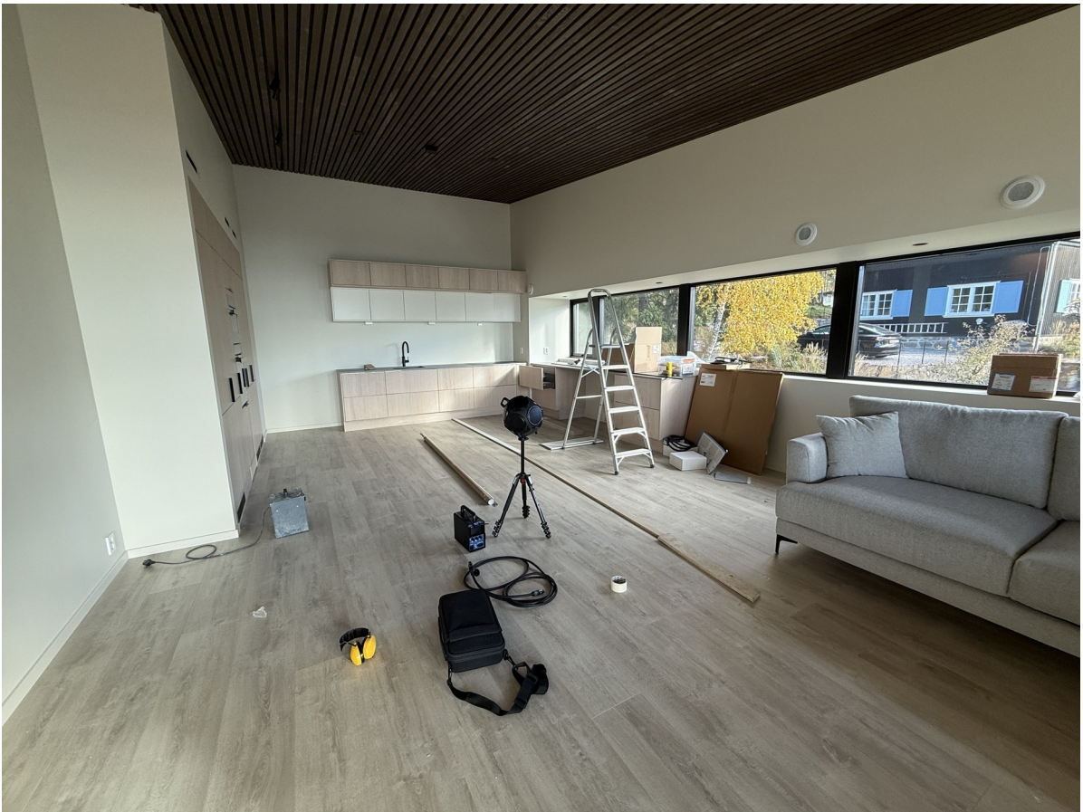
The main dwelling's living room/kitchen with measurement equipment. This is the receiving room for the airborne test.
